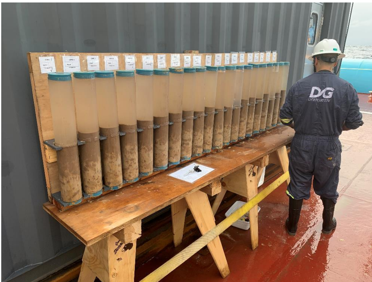
Figure 5-33. Sediment cores from NORI-D showing sediment colour changes and mottling.
