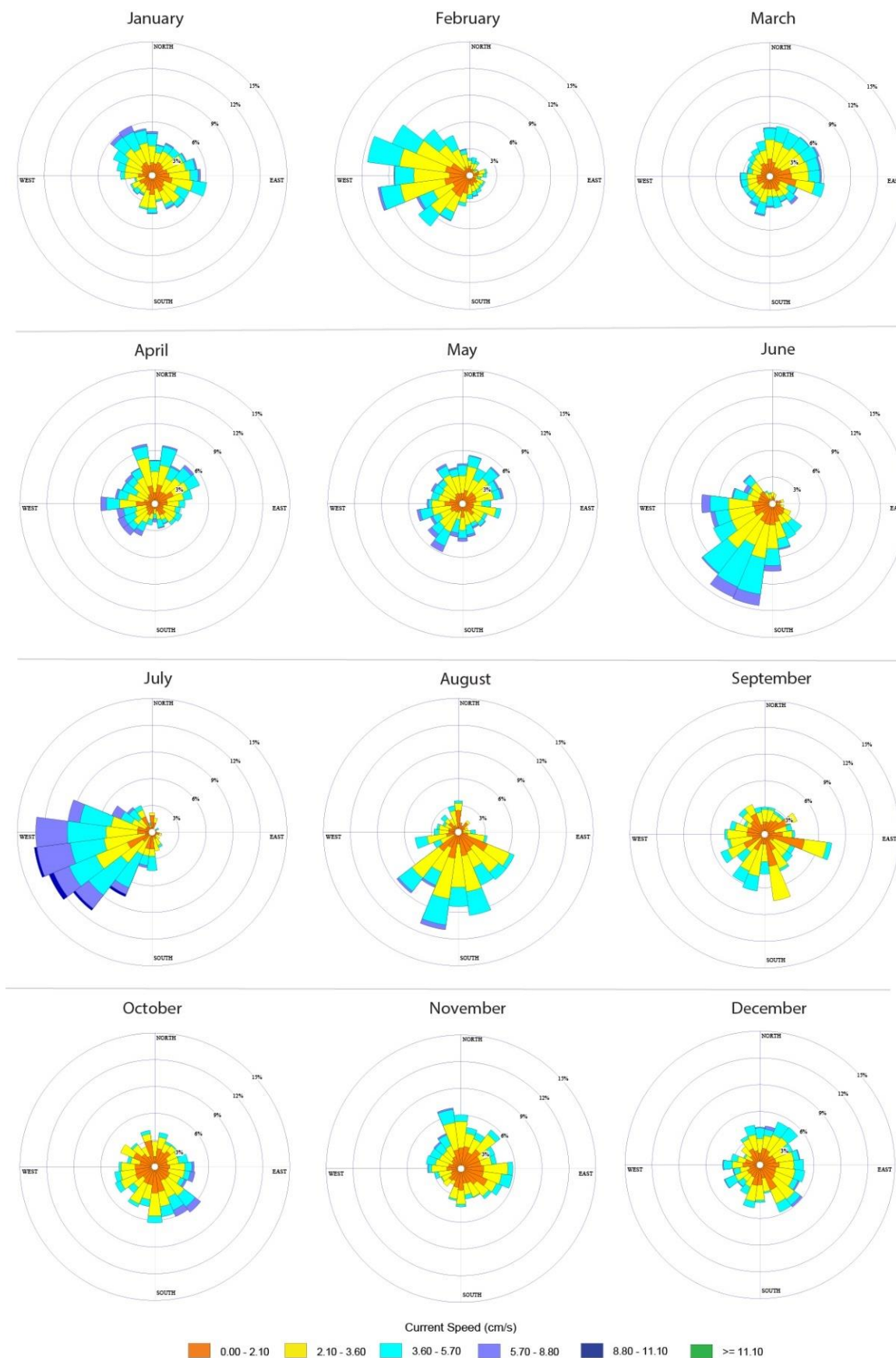
Figure 5-24. Monthly current rose direction (flowing towards) and speed (cm s -1 ) plot recorded from bin #4 of upward-looking acoustic Doppler current profiler (ADCP) (300 kHz) at 2,000 m on the Long Mooring between 15 October 2019 and 2 June 2021.
