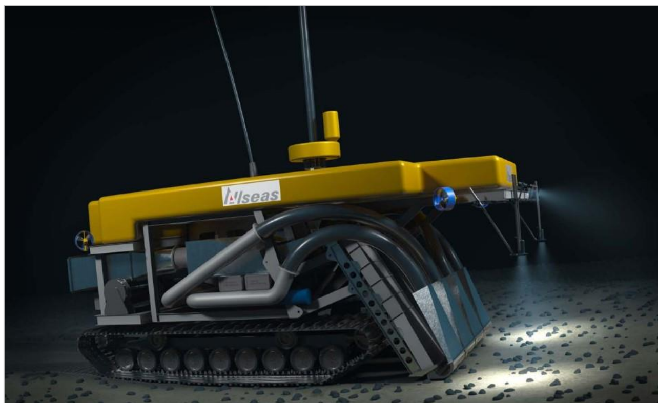
Figure 3-7. Rendering of Prototype Collector Vehicle
