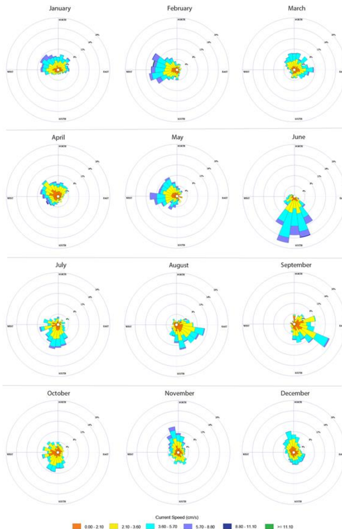
Figure 5-28. Monthly current rose direction (flowing towards) and speed (cm s -1 ) plot recorded from bin #4 of the downward-looking Acoustic Doppler Current Profiler (ADCP) (600 kHz) at 4,321 m water depth. (i.e., 5 m above the seafloor) on the Long Mooring between 15 October 2019 and 24 April 2021.
